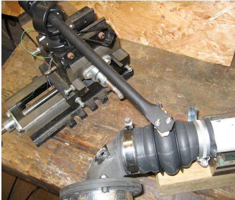
Figure 2, record player arm used to measure the vibration at a point on a hose
